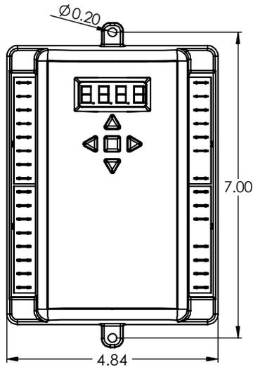
**Figure 4: DFC+ Side View with dimensions (inches)**
